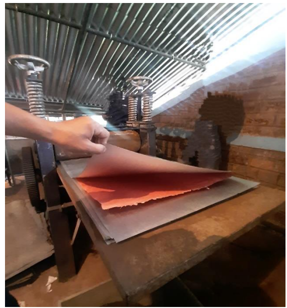
Fig:Paper under Calendering process
