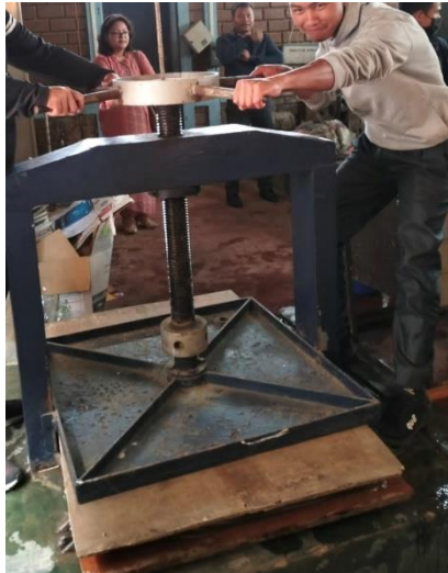
Fig: Drying in Screw Pressing
