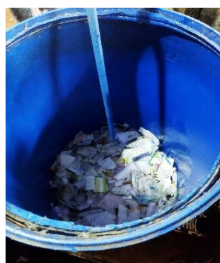
(b) Mixing the waste paper with water
